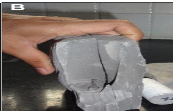
Figure 5A:A fractured core plug B.A fractured sample while retrieving in the core plug
