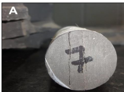
Figure 5A:A fractured core plug B.A fractured sample while retrieving in the core plug
